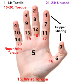
Figure 3: Tactile functional-area definition of MTTS.
