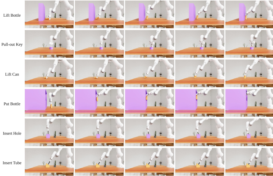
Figure 11: Representative rollouts on the UniVTAC simulation benchmark. Each row corresponds to one task and shows five key frames from a rollout.
